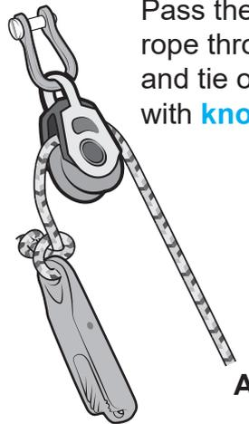
d) Tie off the long piece of rope onto the bottom of the clam cleat with **knot #1**.
