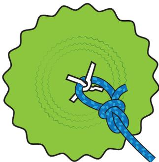
Run the downhaul line up the sail and tie it off on the upper patch (onto the cross of webbing) with **knot #2**.
