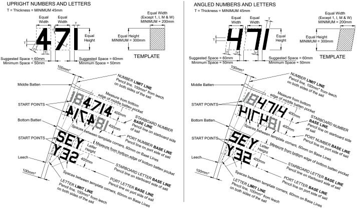
1. MINIMUM SPACE BETWEEN NUMBERS AND LETTERS IN THE CLASS RULES IS 50mm, SO USE 60mm TO ENSURE THAT ANY SMALL ERRORS IN POSITION ARE STILL LEGAL. 2. LAST FOUR DIGITS OF SAIL NUMBER TO BE ONE DARK, DISTINCTIVE COLOUR OR BLACK. PRECEDING DIGITS TO BE A DIFFERENT, CONTRASTING, DISTINCTIVE, COLOUR, PREFERABLY RED. ALL NATIONAL LETTERS TO BE ONE COLOUR. THEY MAY BE ONE OF THE COLOURS OF THE SAIL NUMBER DIGITS OR ANOTHER DISTINCTIVE COLOUR.
